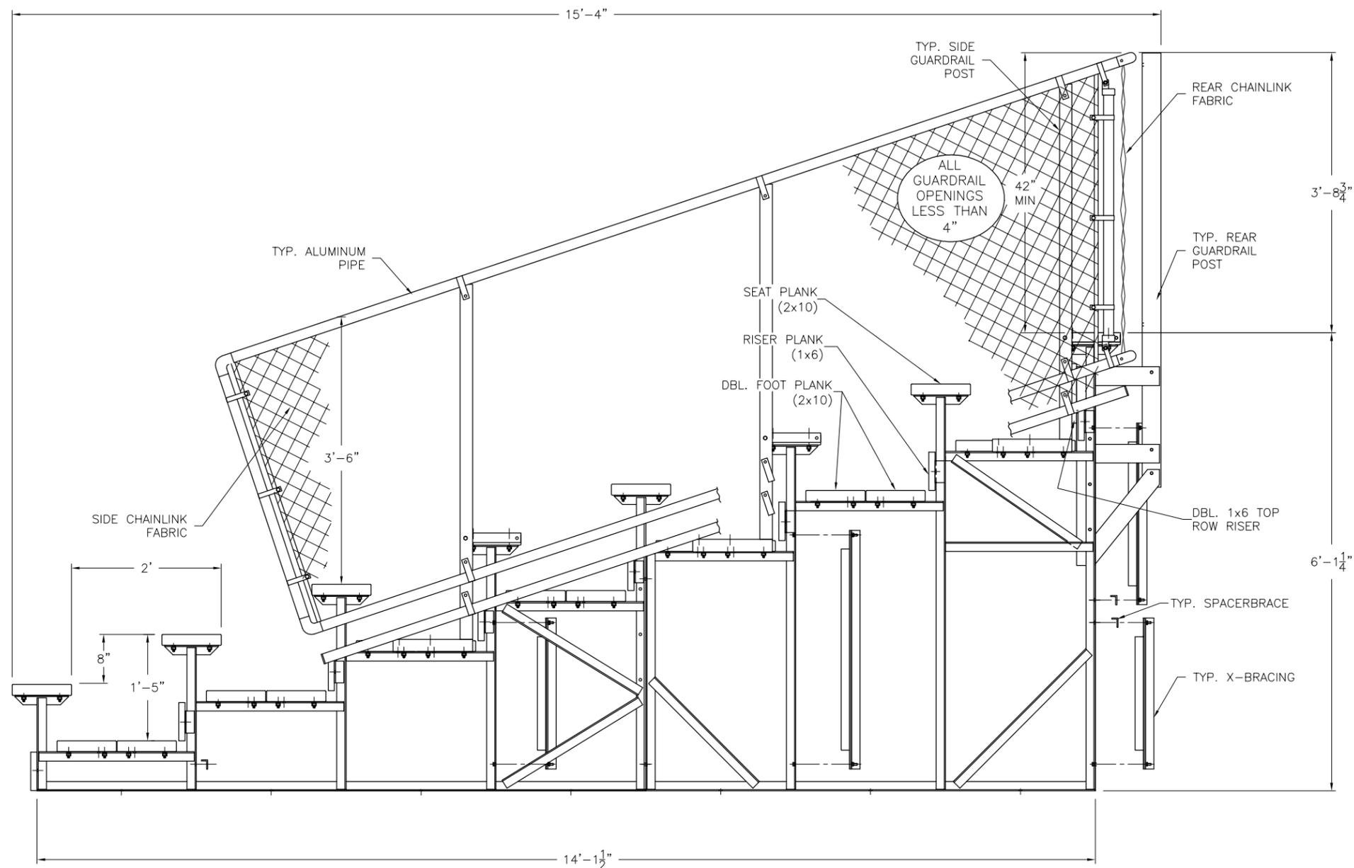
**NOTE:** ILLUSTRATION SHOWN WITH DOUBLE FOOT PLANK, 1x6 RISER (ROWS 1-7), DBL. 1x6 RISER (ROW 8), & CHAINLINK GUARDRAIL. PLEASE REFER TO ATTACHED SPECIFICATIONS FOR FEATURES INCLUDED WITH YOUR SPECIFIC BLEACHER.
