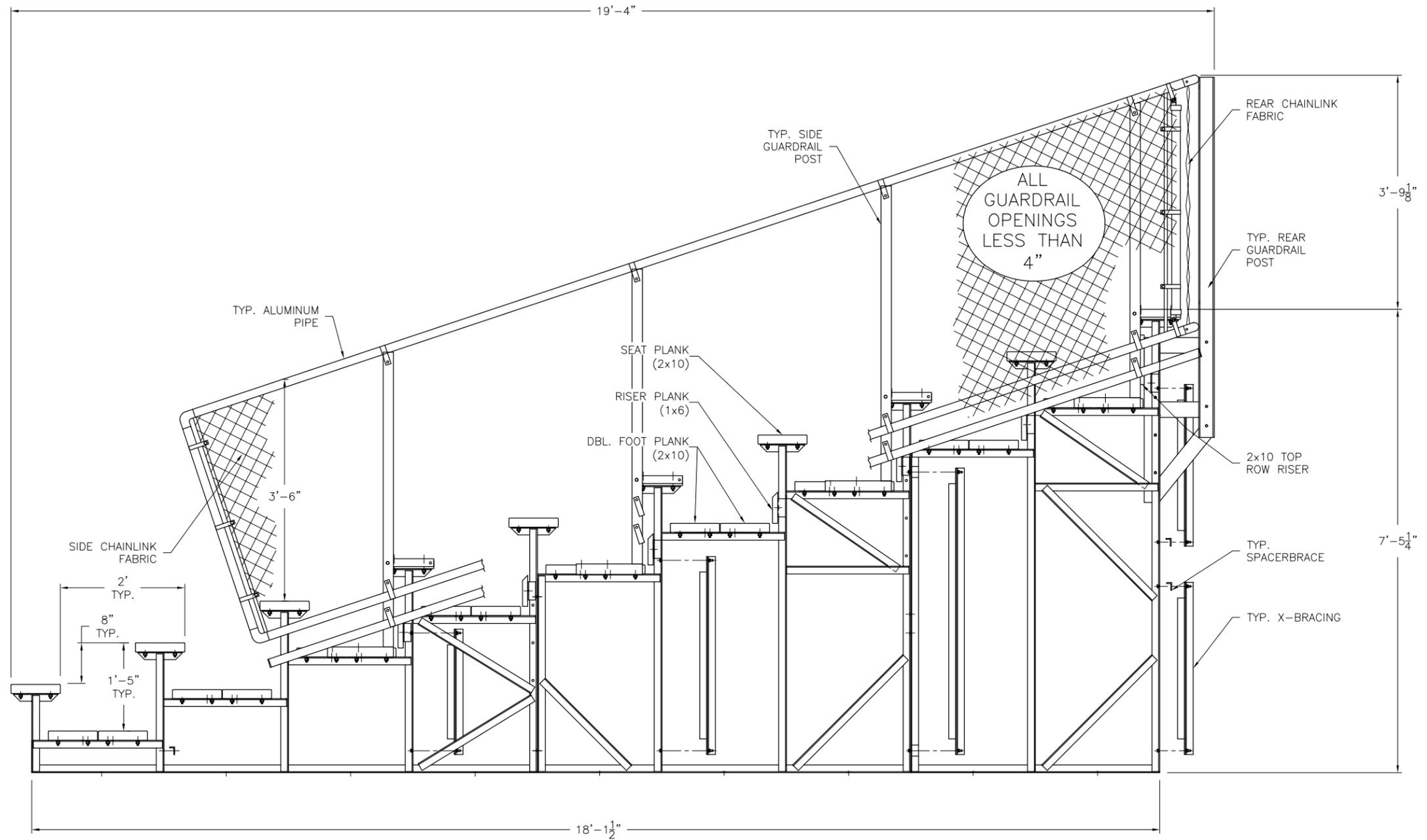
**NOTE: ILLUSTRATION SHOWN WITH DOUBLE FOOT PLANK, 1x6 RISER (ROWS 4-9), 2x10 RISER (ROW 10), & CHAINLINK GUARDRAIL. PLEASE REFER TO ATTACHED SPECIFICATIONS FOR FEATURES INCLUDED WITH YOUR SPECIFIC BLEACHER.**
