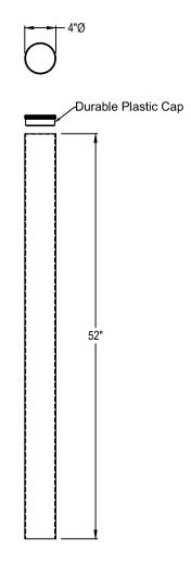
Ground sleeves shall be constructed out of a 4" outside diameter steel tube with a galvanized finish and have an interior diameter of 3 19/25". Product is 52" long providing for depth in a sand volleyball court and proper drainage. A durable plastic cap is provided to keep sand out. Installation to be completed in accordance to manufacturer's instructions. Do not scale drawings. Each sleeve shall weigh approximately 35#.
