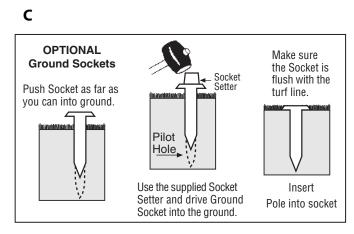
**STEP 5:** With the 1st pole installed, PULL TIGHT on the 2nd sleeved pole to mark the optimum location on the Radius Line (see X noted below) ... create pilot hole, install the pole or socket as per STEP 4... keep repeating this process for remaining support poles.
