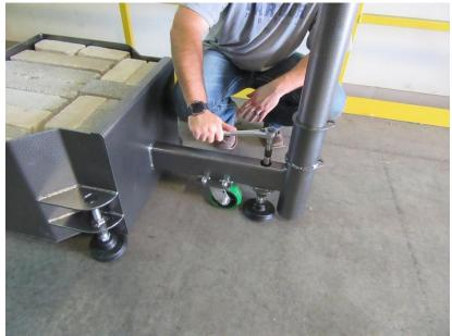
5. Next, lower the STABALIZER FOOTPADS down until they touch the floor on both the left and right sides of the ballast box as shown below.
