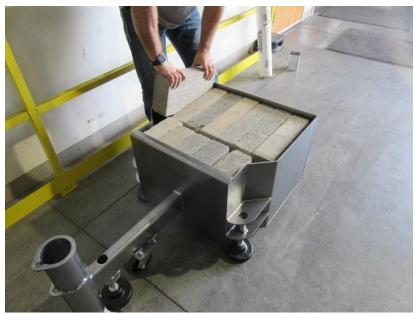
4. Using a socket wrench with extension and  $\frac{3}{4}$ " socket, lower the FRONT FOOTPAD onto the floor so the caster wheel is approximately  $\frac{1}{4}$ "- $\frac{1}{2}$ " off the floor.
