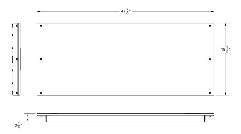
NOTE: As with all wooden take-off boards, if allowed to sit in standing water the board will eventually swell. This condition can cause permanent damage to the board. To maximize service life, runway recesses for take-off boards should be drained. The seat plank base elevates the board from the bottom of the tray - providing 1 3/4" clearance from standing water.
