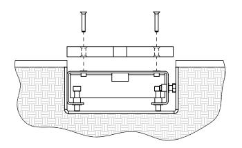
Replace the Take-Off board (44404) and secure it in place with four screws (M2257).
