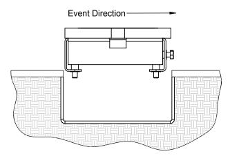
Place the Take-Off & Base Board Assembly (44410) in the Tray (443) so that the locking blots (M2787) face the sand pit.
