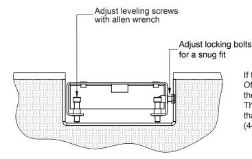
If the board needs adjusting, remove the Take-Off board (44404) and an allen wrench to adjust the leveling screws (M2530) from the top down. The locking bolts (M2787) can be adjusted so that the base board (44402) sits tight in the tray (443).
