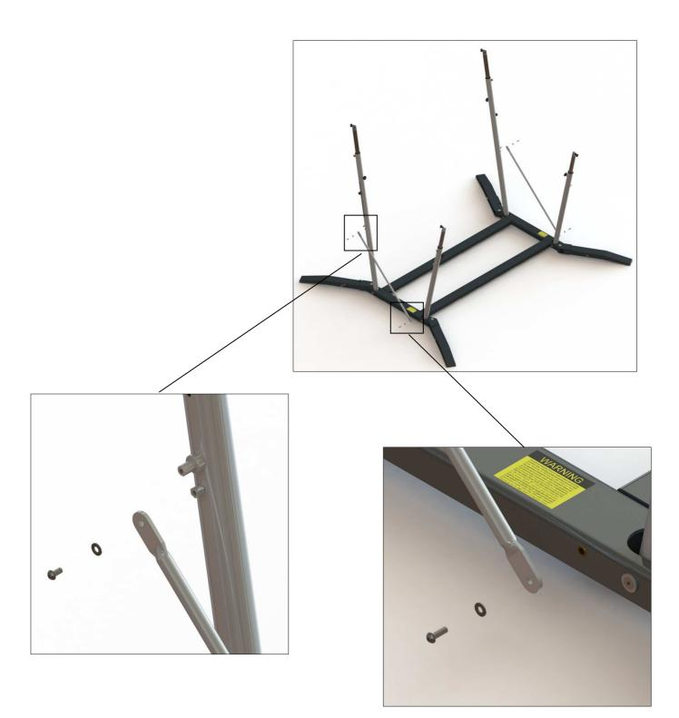
In order to mount the diagonal distance interlock to the high upright, use a M10x20 button head bolt (incl. Loctite sealing) with a washer M10 and for mounting it to the lower upright, use a M10x25 button head bolt (incl. Loctite sealing) with a washer M10.
