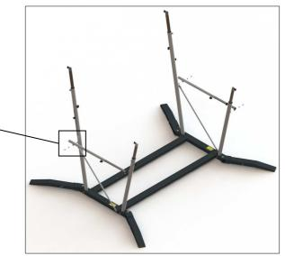
Mount the width adjuster to the uprights using button head bolts M10x20 with washers M10 and fasten them tightly.
