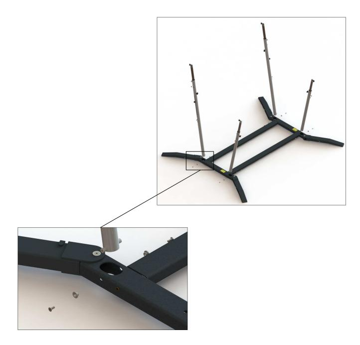
Lay the base frame on a flat surface and carefully place the uprights in the therefore designed cavities.
