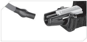
To change resistance cables, open Slide-Lock door (A) by pushing up from bottom. At approximately a 45° angle, thread the end of the cable all the way through opening before sliding the door back down.
