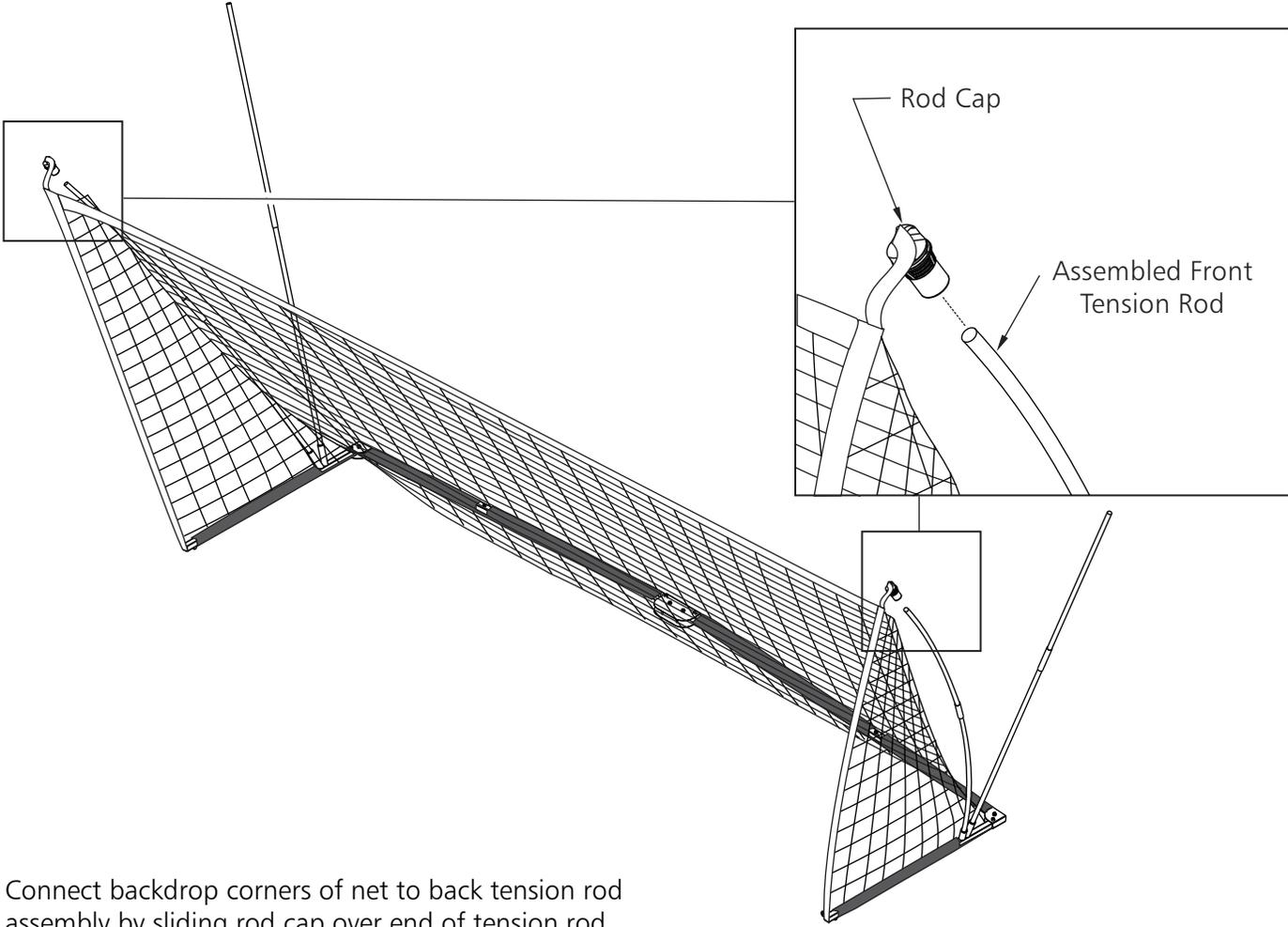
7. Connect backdrop corners of net to back tension rod assembly by sliding rod cap over end of tension rod.
