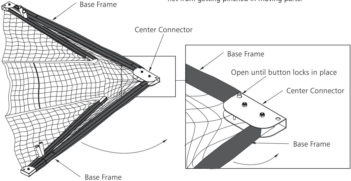
3. Pull left and right rear base until button locks into place on right and left center base. **Do not force parts.** Parts should move freely, if parts do not, look for points where net may be caught on frame.
