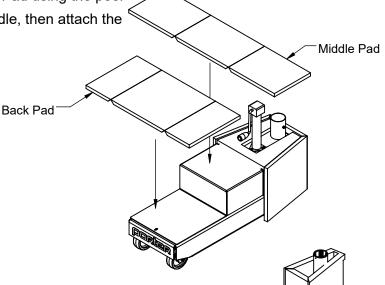
7. Attach the Top Pad with peel and stick Velcro. Finish pad installation by attaching the Pole Pad.
