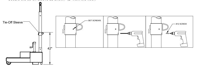
3. Attach the winch (WINH00113) 42" from the floor using the instructions provided in the winch box
