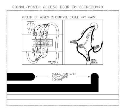
2. The connections are standard black, white, and green (ground). Replace the cover when complete.
