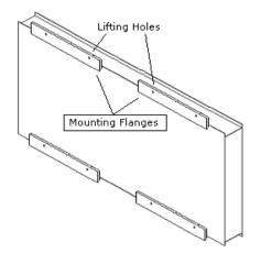
2. Lift the scoreboard into place to the desired height, ensuring that the scoreboard is level.
