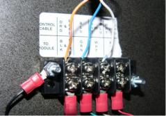
NOTE: Refer to the connections that were made at the scorekeeper's location. Make the connections at the scoreboard match the connections at the scorekeeper's location.
