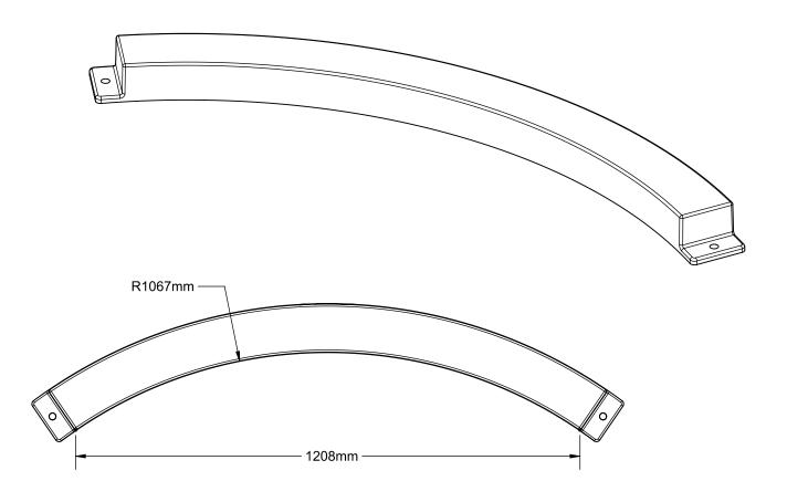
The 363 Cast Aluminum Toeboard is designed to be used with a 3/4" [19mm] depressed throwing surface formed by an aluminum shot circle embedded in the concrete pad.
