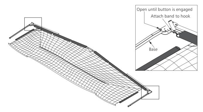
5. Add one tension rod w/coupler to each base through net sleeve on sides of net.
