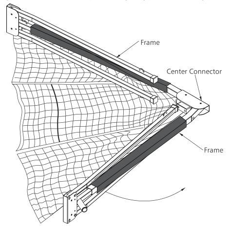
3. Extend rail sections by pulling on each base connector until buttons lock into place. <u>Do not force parts.</u> Parts should move freely, if parts do not, look for points where net may be caught on frame.
