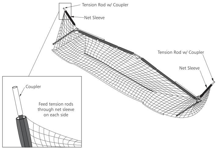
6. Tilt frame towards the unopen bases to add remaining tension rods. Attach net attachment loops to net attachment points on poles.
