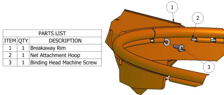
Figure 5-6: Screw net attachment ring to rim.
