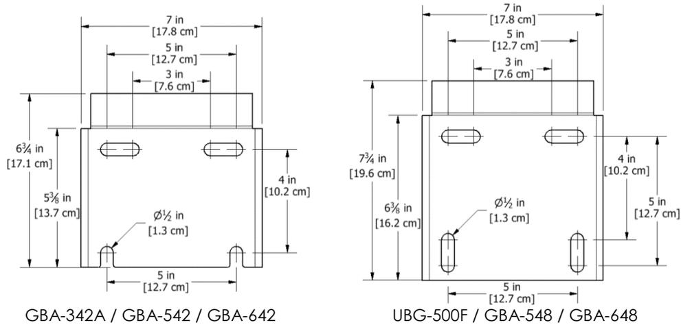
Figure 2-1: Mounting bolt patterns.
