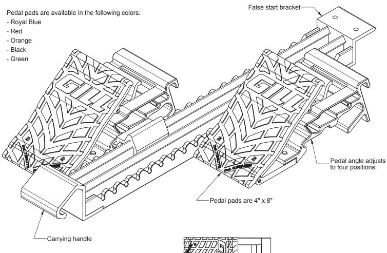
Precise and consistent foot placement is ensured using the integrated pedal markings. Pedals are adjustable to 30°, 40°, 50°, and 60° settings. Angled spikes in the base of the pedals guarantee a start with absolutely no slipping. Built in handle allows for easy carriage.
