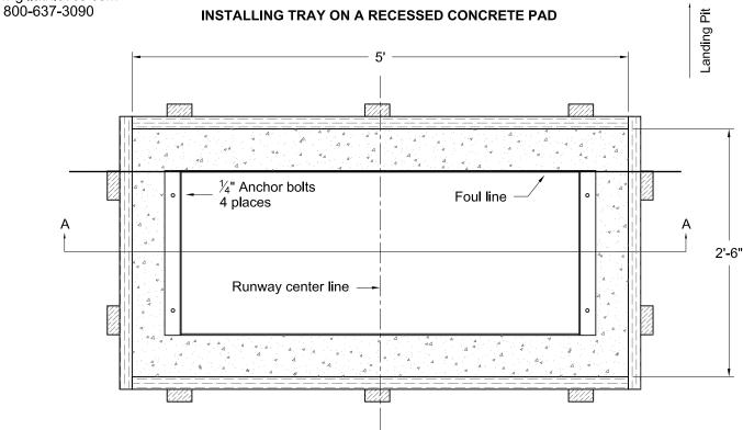
When positioning tray on base concrete, insure tray sits flat and does not warp when anchored in place. The tray lid should not rock if tray is properly installed. When finishing runway subsurface around the sides of the tray, insure the procedure does not deform the tray sides inward.
