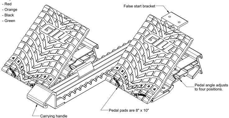
Precise and consistent foot placement is ensured using the integrated pedal markings. Pedals are adjustable to 30°, 40°, 50°, and 60° settings. Angled spikes in the base of the pedals guarantee a start with absolutely no slipping. Built in handle allows for easy carriage.
