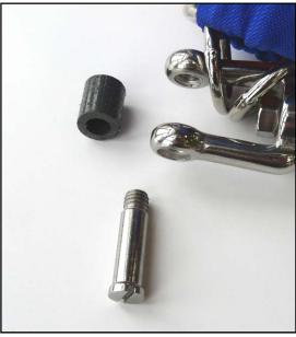
2. Slide the rings of the harness into the swivel yoke. While re-installing the threaded pin, place the spacer between the yokes and run the pin through it. Tighten down the threaded pin.
