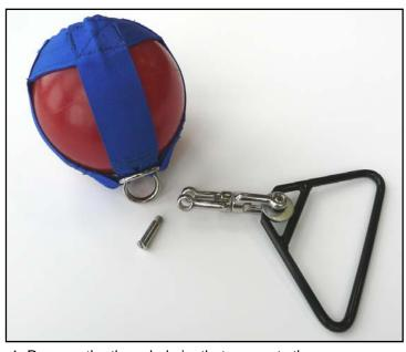
1. Remove the threaded pin that connects the swivel to the rings on the harness.
