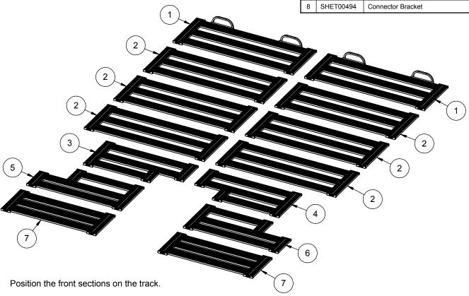
Lift up the back and place the Connector Brackets under the planking. Use two brackets per section; one at each end.
