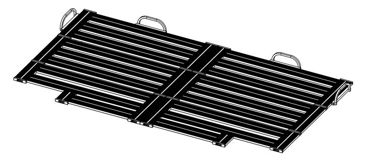
Made of corrosion-resistant aluminum, this platform supports the 646 high jump landing systems above the ground to prevent water damage. The platform consist of individual, easy to carry and convenient to store pallets which are quickly assembled and disassembled.
