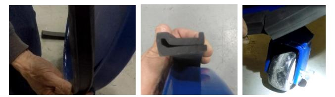
Once installed, one end of the new rubber should touch the other end, you can gently stretch the rubber as you wrap it around the base. You can have a maximum ¼" gap (end to end) after it is installed on the base. It is best if each end is touching.
