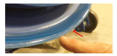
It is most important to make sure between that the two wheels, the inside edge and lip of the base is very smooth.
