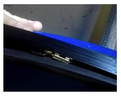
16. Attach the screw clamp as shown. Please make sure that the writing is facing up on the band clamp because the direction this pulls is important. Trim the band to the correct length once you are sure of the amount of wire needed. That will be the size you will need for the rest of the bases you are repairing.
