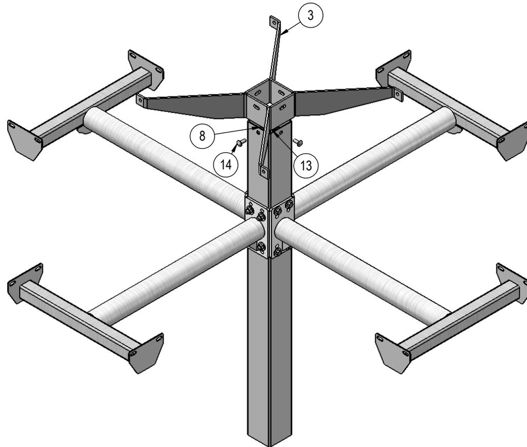
Attach the H Bracket to the 338 Post using specified hardware.
