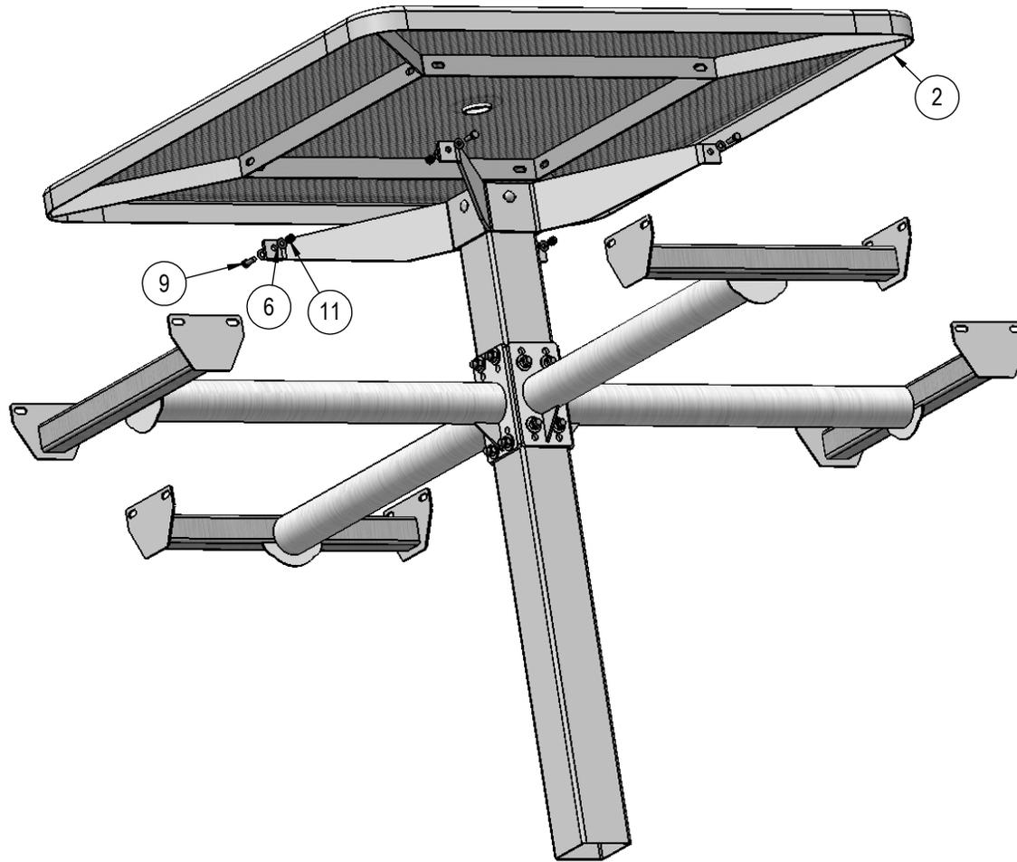
Attach the 46" Square Top to the H Bracket using specified hardware.
