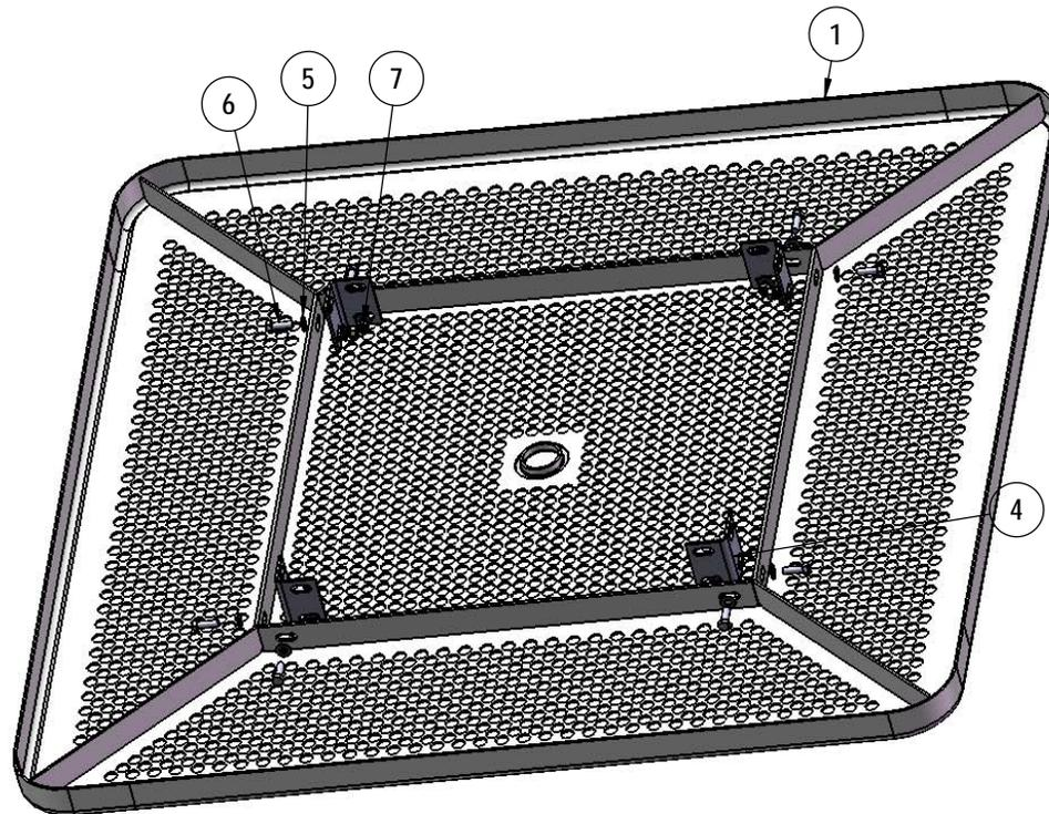
Attach the 358 Extension Tabs to the 46" Table Top as shown using specified hardware.
