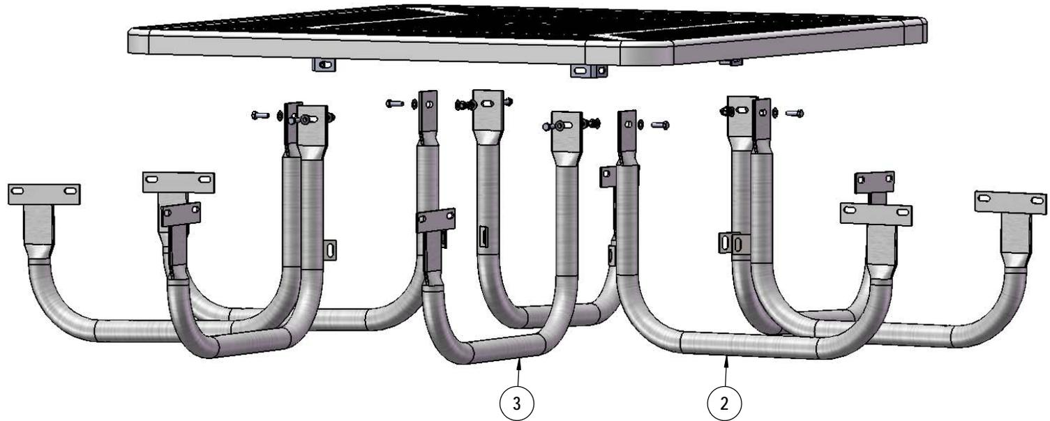
Attach the 358 Legs to the Extension Tabs as shown using specified hardware.
