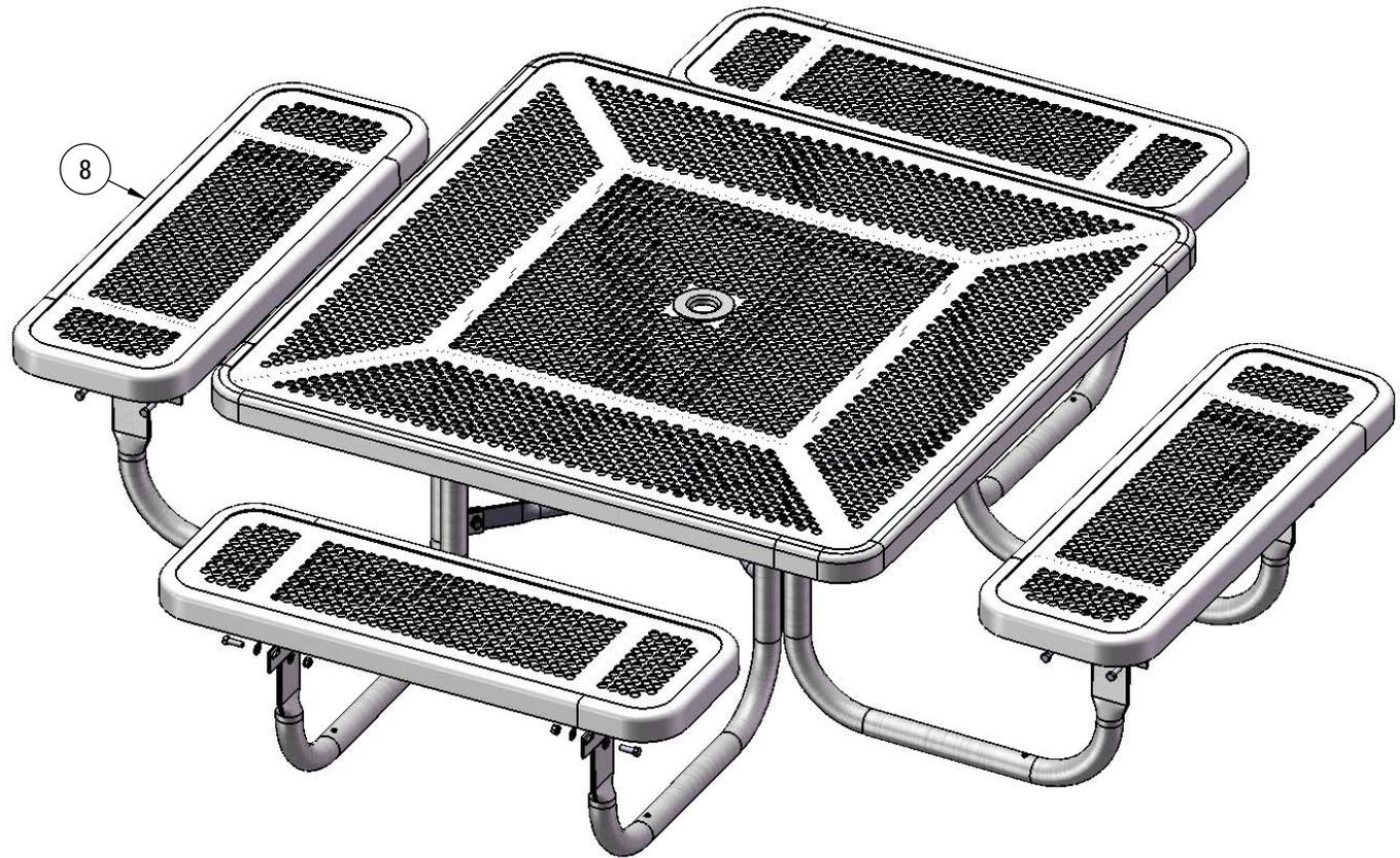
Attach the 3' Seats to the Legs as shown using specified hardware.
