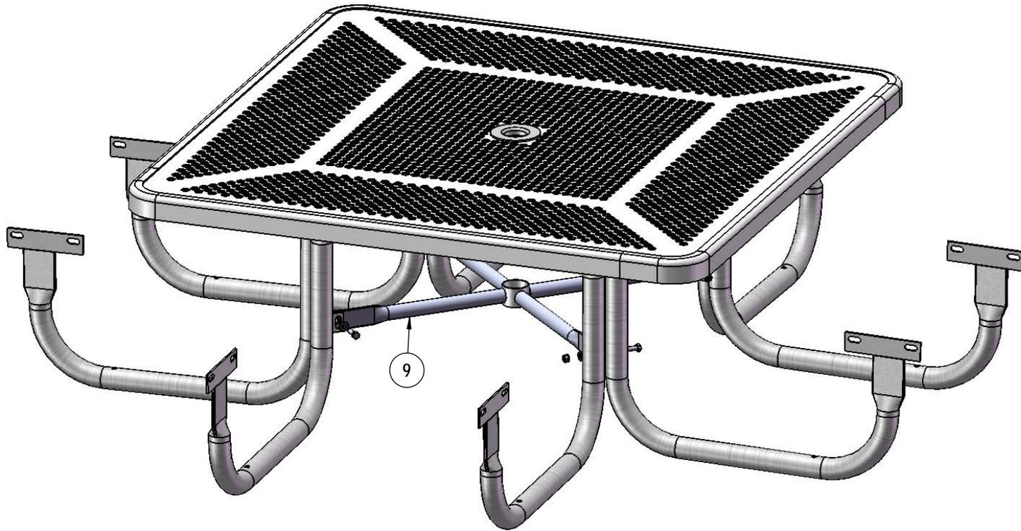
Attach the 358 Crossbrace between the Table Legs as shown using specified hardware.
