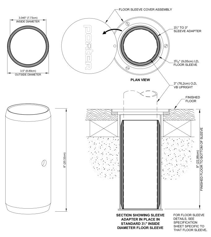
\_ - 00827-300 FLOOR SLEEVE ADAPTER FOR 3" DIA. UPRIGHT IN 3½" DIA. SLEEVE
