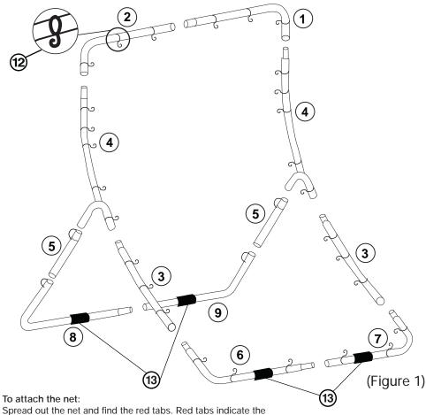
corners. Start by attaching all of the corners of the net to the frame with the bungees and then proceed with the sides of the net until all bungees are secure.
