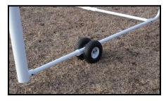
**Step 1:** Face both tires inward toward the carriage. Slip both bolts inside the wheels. Fasten each wheel to the carriage using the 4 axle bolts. Ensure wheels are installed. Make sure valve stems are facing outward. Tighten all bolts securely.
