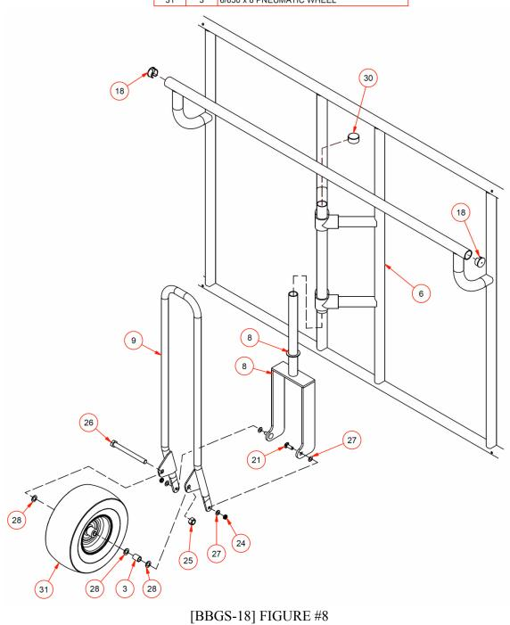
After the frame is fully assembled check all hardware to make sure it is tightened and all joints are secured. Raise the upper frame arches into position, using the strut pipes, and check for alignment. (See setup instructions)
