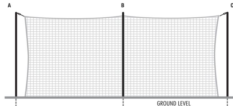
Ropes attach to the hanging-loop assemblies on crossbars A, B, and C.
