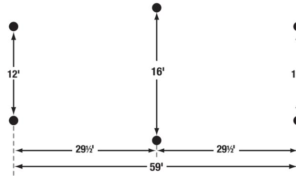
**4.** SIDE VIEW OF THE THREE U-SHAPED SECTIONS COMPLETELY SET UP.
