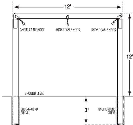
**2.** Once you assemble it, the middle section will look like this. Insert a short hanging-loop assembly into the middle pre-drilled crossbar hole and long hanging-loop assemblies into both outside pre-drilled crossbar holes.
