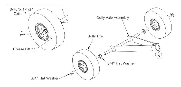
5. Complete the assembly of dolly as shown but do <u>NOT</u> tighten bolt until all parts are attached. Note the orientation of holes in dolly handle.
