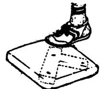
Step 7: Step on cover until it completely snaps over the tee and lays flat on the ground. The ground below the base cover should be flat and level with no hollows, depressions, or buildup under the base.
