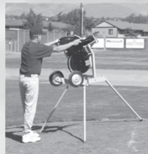
Figure 4 Carefully tilt Junior Hack Attack up onto its rear legs
