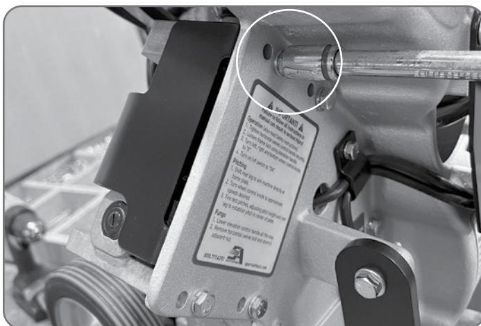
Figure 9 Shown using a 6" extension with 1/2" socket.
