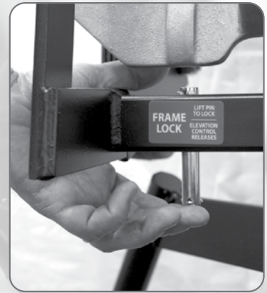
Figure 8A Push up frame lock pin
