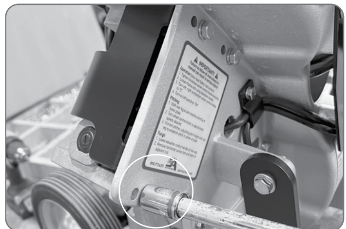
Figure 10 Shown using a 6" extension with 7/16" socket.
