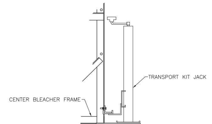
PLACE JACK ON UNDER SIDE OF HORIZONTAL BRACE APPROX. 14"-18" AWAY FROM CENTER FRAME, AS SHOWN. BLEACHER SHOULD ALWAYS BE ON SOLID, LEVEL GROUND, AND BE STABILIZED TO PREVENT MOVEMENT WHEN USING JACK.
