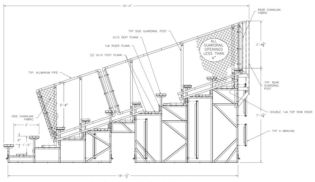
NOTE: ILLUSTRATION SHOWN WITH SINGLE FOOT PLANK ON ROWS 2-3, & DOUBLE FOOT PLANK ON ROWS 4-10, 1x6 RISER ON ROWS 4-9, DOUBLE 1x6 RISER ON ROW 10, & CHAINLINK GUARDRAIL. PLEASE REFER TO ATTACHED SPECIFICATIONS FOR FEATURES INCLUDED WITH YOUR SPECIFIC BLEACHER.
