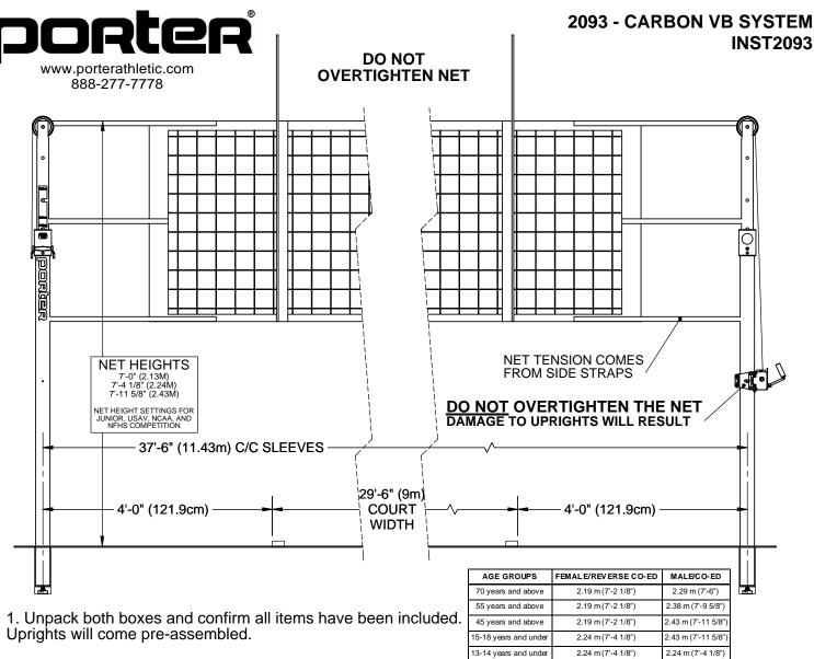
2. Place assembled standards into floor sleeves. Rotate until the 11-12 years and under winch and tie-off sleeve are oriented as shown above.
