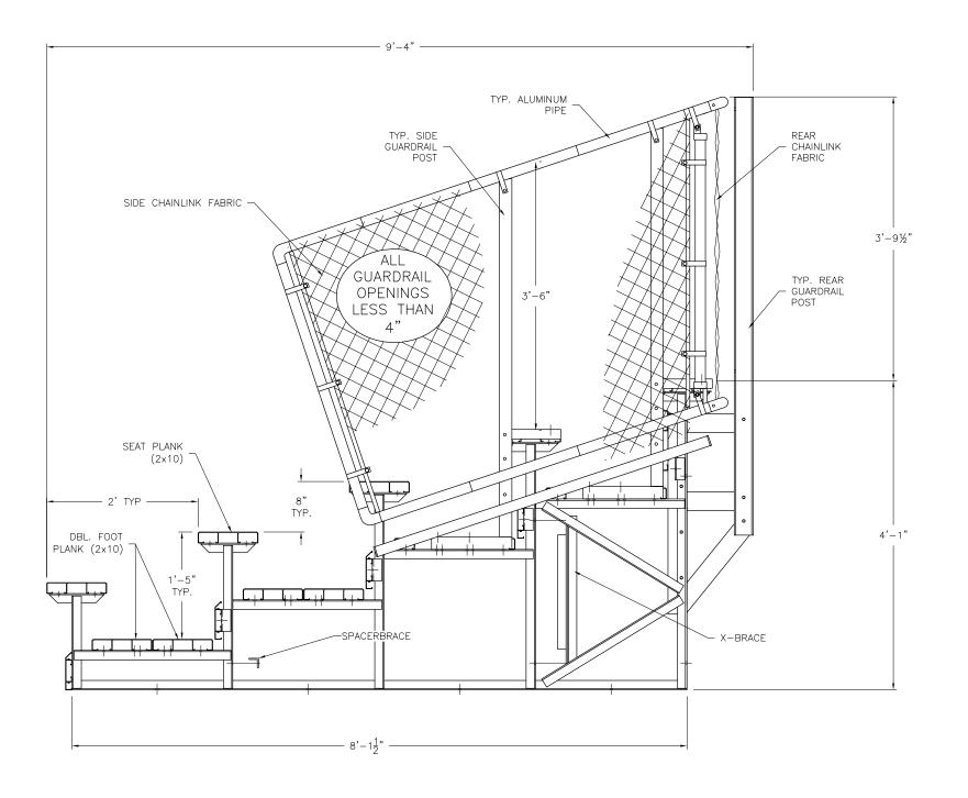
**NOTE:** ILLUSTRATION SHOWN WITH DOUBLE FOOT PLANK, 1x6 RISER (ROWS 1-4), 2x10 TOP ROW RISER, & CHAINLINK GUARDRAIL. PLEASE REFER TO ATTACHED SPECIFICATIONS FOR FEATURES INCLUDED WITH YOUR SPECIFIC BLEACHER.
