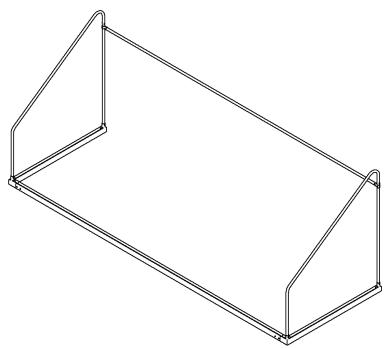
Attach rear crossbar into tee fittings on backstays. Use hardware detailed on assembly drawing. Now tighten all hardware. With goal in the face down position attach the net using the "Easy Clip" net attachment system. If the net is installed in this position, there is no need to climb a ladder and attach netting. Once complete, move the goal into the playing position. **Repeat for the other side**.
