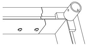
Slide corners into uprights and crossbars. Attach hardware as shown in assembly drawing.
