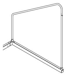
Insert backstays into hubs. Use hardware detailed on assembly instructions.
