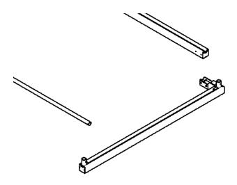
Lay goal components face down in the order they appear on the assembly drawing. This order of construction will make the construction of the goal safe and efficient. Make sure that you have all of the pieces listed on the assembly instructions.
