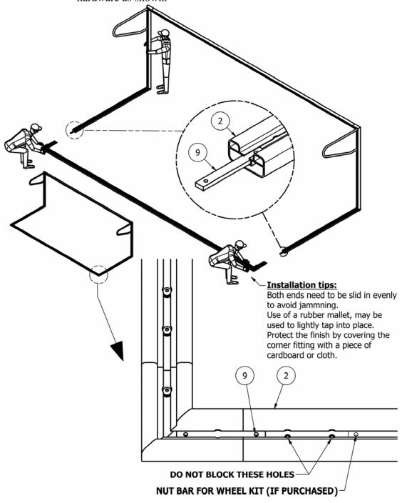
6. Install auxiliary soccer backstay, line up nut bar. Note if the plates don't line up, flip the auxiliary soccer backstay. Install hardware loosely; once parts are aligned tighten all hardware.
