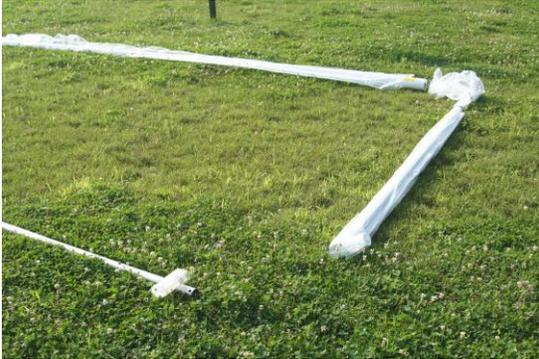
Lay goal components face down in the order they appear on the assembly drawing. This order of construction will make the construction of the goal safe and efficient. Make sure that you have all of the pieces listed on the assembly instructions.
