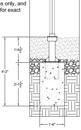
The concrete must be allowed to fully cure before installing the ground sleeves.
