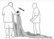
1. Hold Black hinges and place Orange Pocket on ground with Net spread out away from you. Then open frame laying both sides on ground
