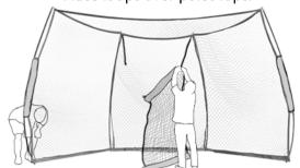
9. Stake the Net to ground via Bungees, Finally attach either baffle to protect backstop.
