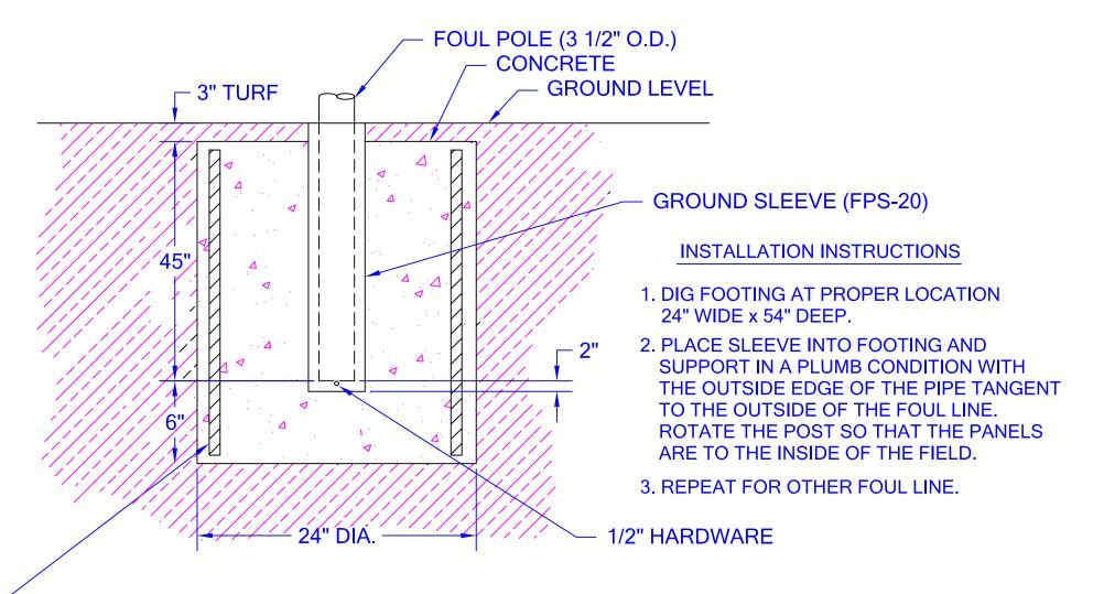
3/4" RE-BAR x 46", 6 PLACES PER FOOTING (NOT INCLUDED, TO BE PROVIDED BY INSTALLER). THESE ARE TYPICAL FOOTING DIMENSIONS FOR AVERAGE SOIL CONDITIONS.
