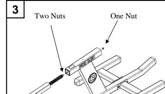
The Mod Ram Unit comes with (3) nuts on the threaded rod at the end of the spring. Remove (2) nuts to use later. Install the Mod Ram Unit by inserting it spring side first into the Ram Outer Tube. The threaded rod on the end of the spring fits through a hole at the back of the head unit. A screwdriver can be used to guide the threaded rod through the hole. Use the nuts you removed earlier to secure the
