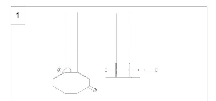
Attach foot pads to leg tubes with (1) 1/2" x 4" bolts and (1) 1/2" lock nuts. Do not over tighten. Repeat for each leg.
