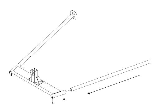
Insert the leg tubes into the beam support assemblies. Position the tops of the leg tubes flush with the tops of the beam support assembly. Secure each leg with (2) 5/8" x 1 1/2" bolts. Repeat for each leg.
