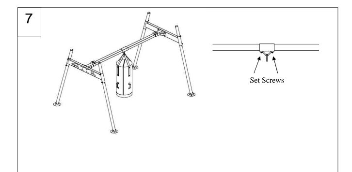
**Double-check to ensure all bolts are tight**. Hang dummy and tighten the set screws to secure to bag in place, set-up is complete. Dummy should be removed when finished using.
