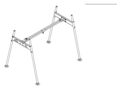
This step will require the use of two or more people. Place the trolley onto the trolley tube with the dummy hanger facing downward. Insert the remaining end of the trolley tube into the second leg assembly and attach same as step 4.
