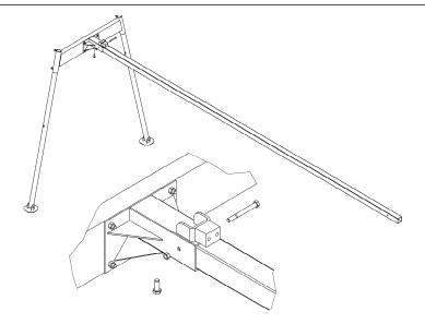
This step will require the use of two or more people. Attach one end of the trolley tube to a leg assembly with (1) 1/2" x 5" bolt and (1) 1/2" lock nut. Also use (1) 5/8" x 1 1/2" bolt to securely tighten trolley beam down.
