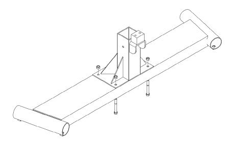
Attach the trolley tube receiver to the beam supports with (4) 1/2" x 4" bolts and (4) 1/2" lock nuts. Repeat.
