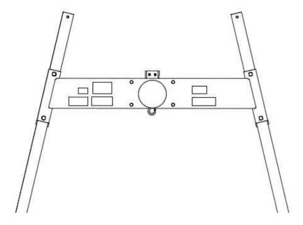
This step will require the use of two or more people. It is possible to vary the slope or height of the assembly by loosening the 5/8" bolts on the leg assembly and raising or lowering as needed. It is recommended that the user lowers one end at a time. Once the desired position is achieved, tighten down all bolts.
