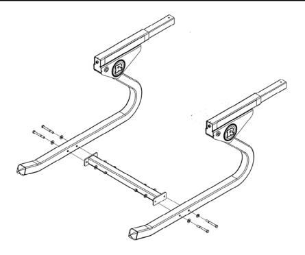
**For 2 man sleds:** Lay Iso Runner Sub Assembly on its side. Connect the runner to the connection link and then stand runner upright to connect the next sled runner. See steps 3 & 4 for ram unit and pad installation. Hardware used for the Connection Links is (4) 5/8" x 6" bolts, (4) 5/8" nuts, and (8) 5/8" washers per Iso Runner Sub Assembly.
