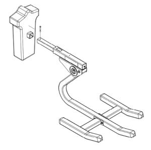
Attach the Surge or Shock pad to the ram unit by sliding pad over ram and inserting fas-pin.
