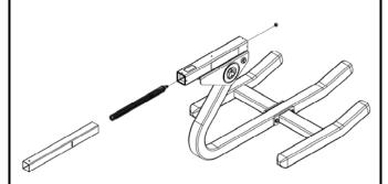
The Lev Ram Unit comes with (3) nuts on the threaded rod at the end of the spring. Remove (2) to use later. Install the Lev Ram Unit by inserting it spring side first into the Lev Head Unit. The threaded rod on the end of the spring fits through a hole at the back of the head unit. Use the (2) nuts you removed earlier to secure the ram in place.
