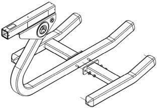
Fit second outrigger over the bolts and secure with (2) more 5/8" washers and (2) 5/8" nuts.
