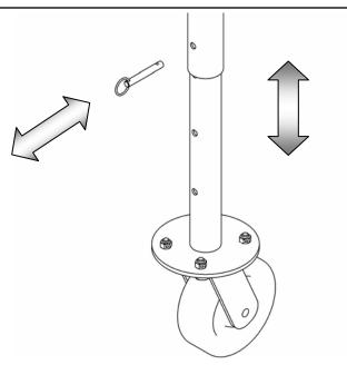
Adjust the height of the Mobility Chute by removing the fast pins from the leg tubes. Raise or lower the tubes to the desired height and reinsert the fast pin. The height can be adjusted from 40" to 69" in 4" increments.
