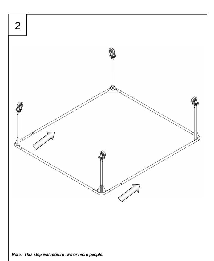
Connect the leg assemblies with the four frame tubes as shown above. Make sure that the leg assemblies are fully inserted into the frame tubes. Once complete, rotate the assembly onto the casters.
