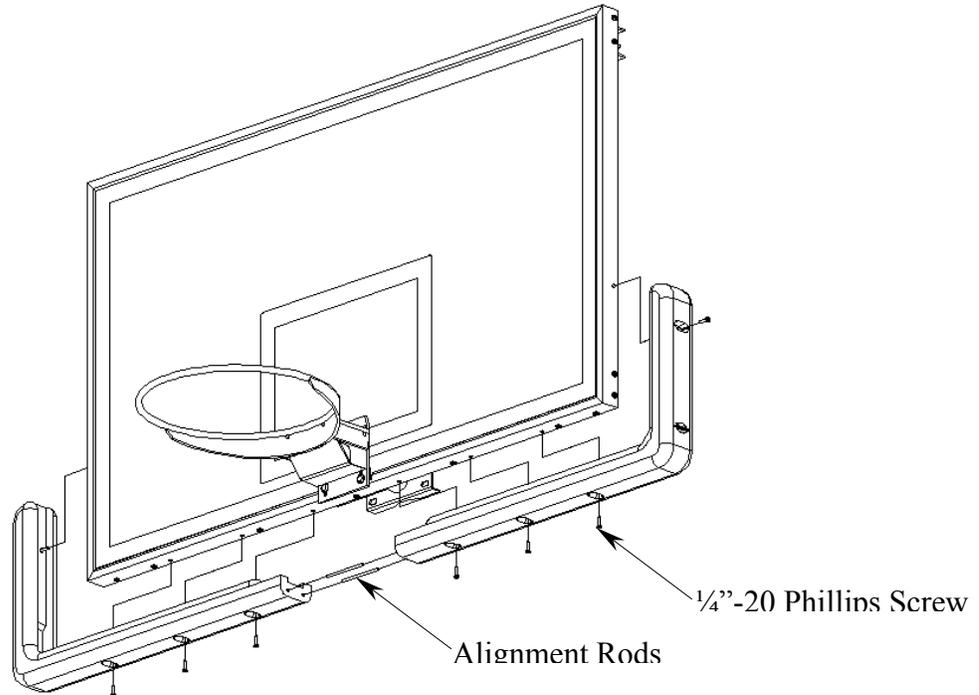
**Figure 2: Assembly of Edge Pad Onto Backboard**
