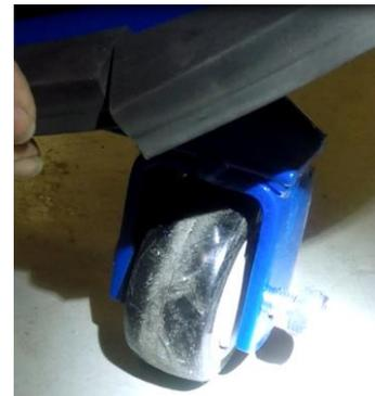
Once installed, one end of the new rubber should touch the other end, you can gently stretch the rubber as you wrap it around the base. You can have a maximum  $\frac{1}{4}$ " gap (end to end) after it is installed on the base. It is best if each end is touching.
