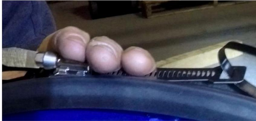
20. Once the band is tight, visually check to make sure the rubber is installed correctly. Test the weighted game standard by tilting the base a few times. If everything looks good you have succeeded.
