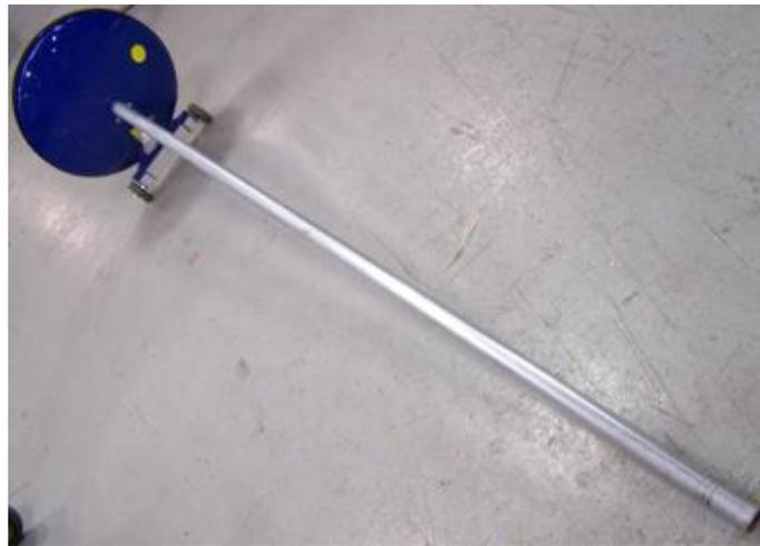
4. Move the base into a position as shown in this picture. Please note the wheels are supported off the ground, the rear part of the base is off the ground and the front of the base is still hitting the ground.
